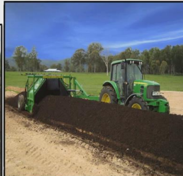
Compost windrow turners are used to mix and stir compost material in commercial agitated composting operations. Source: http://compostwindrowturner.blogspot.com/2017/01/self-propelled-compost-turner.html
